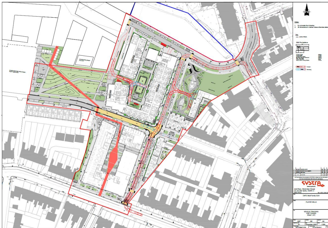
Figure 5.14: Vehicle Tracking for Fire Truck (SYS-PW-04.1)
