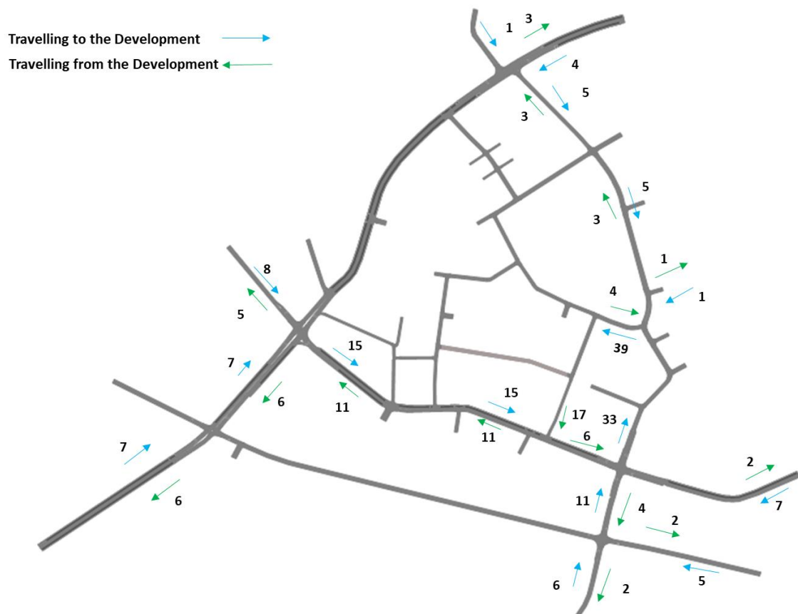
Figure 7.7: PM Peak Development Traffic Distribution
